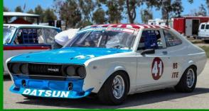
1974 Datsun 710 B-Sedan, \$25,000. Race prepped l20b engine, approx 200hp. Close-ratio 5 speed. LSD. 8point cage. Disc front/drum rear brakes. Coilover front, panhard/leaf/coil rear. Fresh tires, brakes, oils. Ready for the 2019 B-Sedan/Trans-Am 2.5 season. Contact Troy at: racingonthecheap@gmail.com For more info, click here: 710 for Sale
