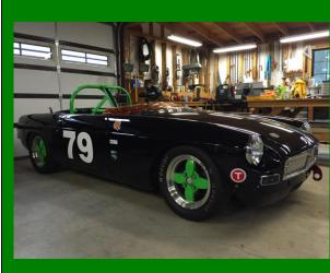
Huffaker prepared MGB - 1800 c.c. w/comp. crank, carrilo rods, J.E. pistons, big valve head, custom 2" header and exhaust, rebuilt carbs, new wires and ignition system. Close ratio dog-ring trans w/2 LSD diffs; 4.55 & 3.90. 2 sets wheels, Accusump & fire system. Spare set adjustable shocks and new Schroth 6 way harnesses.
