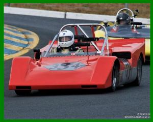
SR4 Bobsy Sportsracer built by Jerry Mong of Medina, Ohio in the 1960's. He constructed two SR4's, this is the only one still racing. The SR4 has a semimonocoque aluminum chassis, fiberglass body, dry sump 1600cc Ford Kent engine w/ twin Webers and a Mk9 Hewland 5-speed gearbox. New engine built by Moore Speed in 2018 with 3 race weekends. Fully documented history with all logbooks. Current owner has raced it on the west coast with CSRG, SVRA, HMSA, and VARA, with additional trips to
